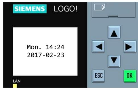
**Step 6:** Exit by pressing the “ESC” key three times. Then press the “OK” key.
