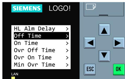
**Step 4:** Press ▲ or ▼ to select the desired parameter to adjust and press “OK”. Continue to **Step 5** on the following pages for the specific block type being edited.
