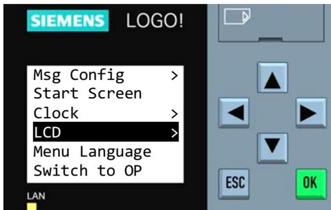
**Step 3:** Press ▼ three times to select “LCD” and then press “OK”.
